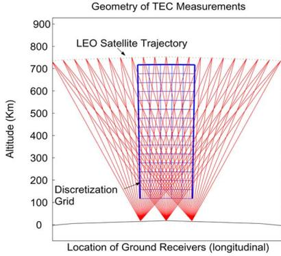
Fig. 1. Typical scenario for ionospheric radio tomography.
