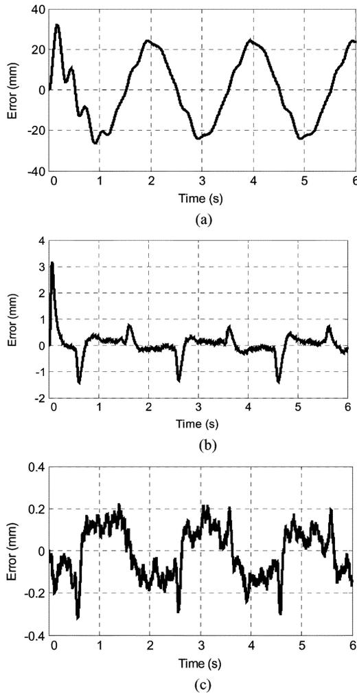
Fig. 9. Tracking errors for sine-wave motion with  $V_{01}, V_{02}$  changes. (a) Without parameter adaptations. (b) ARC-LP. (c) Proposed control (ARC-NP).
