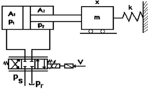
Fig. 1. Schematic diagram of the hydraulic system.
