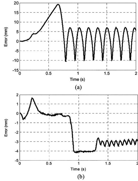
Fig. 5. Tracking errors with  $V_{01}, V_{02}$  changes. (a) Without parameter adaptations. (b) ARC-LP. (c) Proposed control (ARC-NP).
