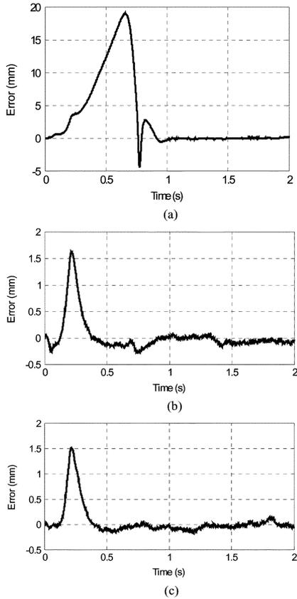
Fig. 4. Tracking errors with no change. (a) Without parameter adaptations. (b) ARC-LP. (c) Proposed control (ARC-NP).
