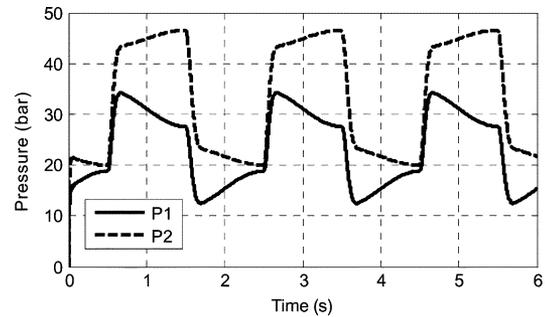
Fig. 10. Pressures in two cylinder chambers for sinusoidal motion with  $V_{01}, V_{02}$  changes.
