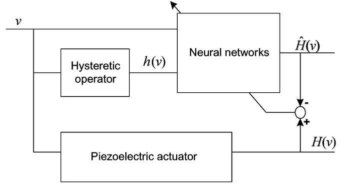
Fig. 3. Schematic diagram of neural networks-based hysteresis model.
