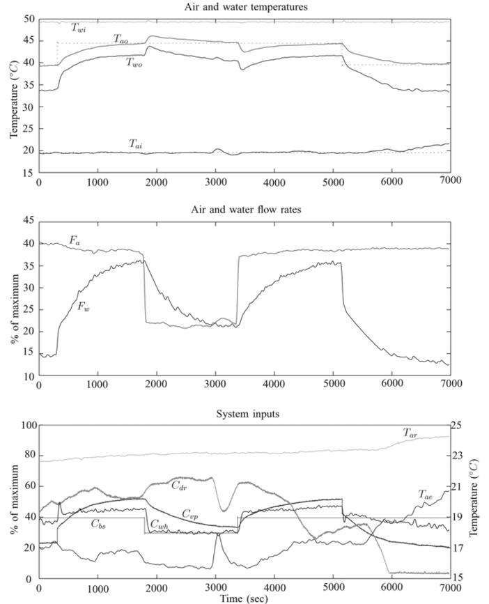
Fig. 6. Controller  $K_{PI}$  experimental test results.
