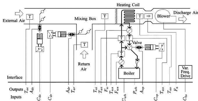
Fig. 2. Diagram of the experimental system and interface signals.
