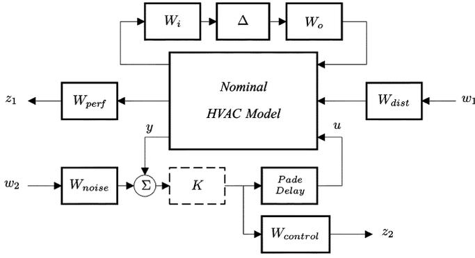
Fig. 3. System model configuration for controller synthesis.
