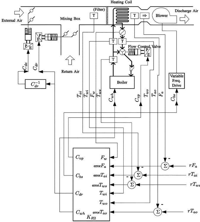
Fig. 5. Experimental system using MIMO robust controller  $K_{R2}$ .
