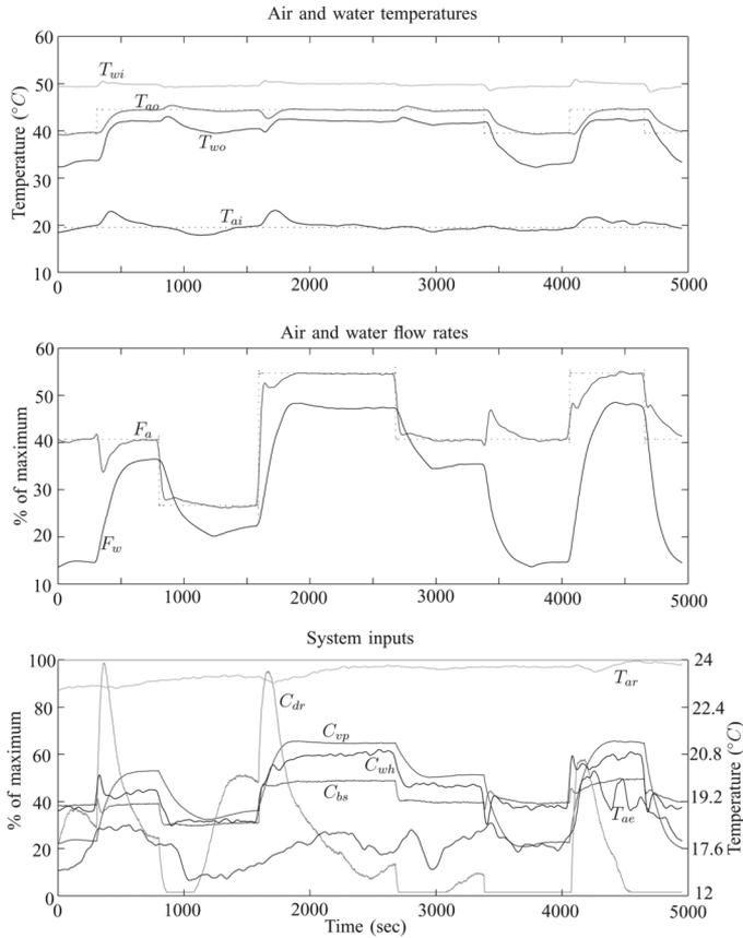
Fig. 7. Controller  $K_{R2}$  experimental test results.
