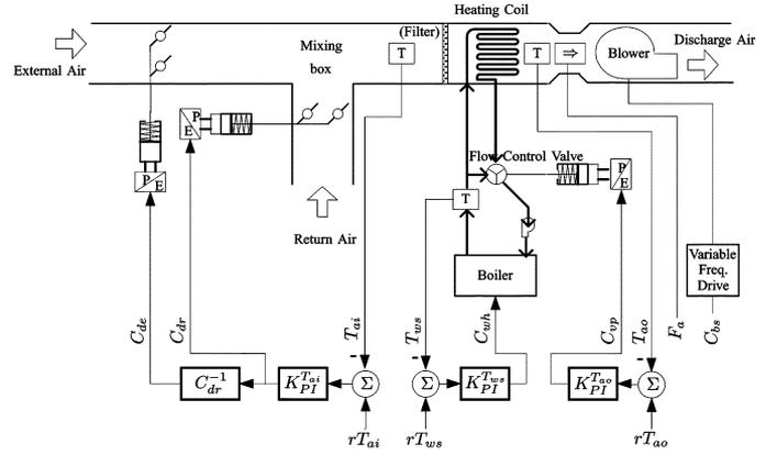
Fig. 4. HVAC controller based on three SISO PI controllers.
