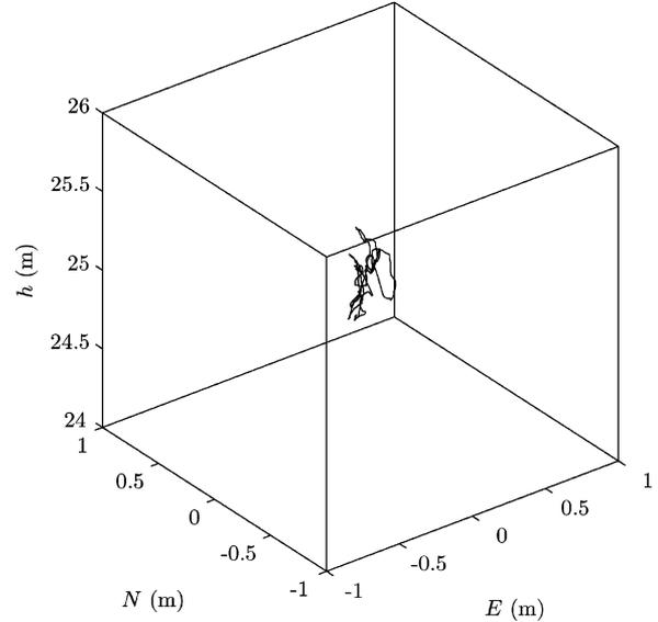
Fig. 11. Airship 3-D position coordinates for turbulent gust case.
