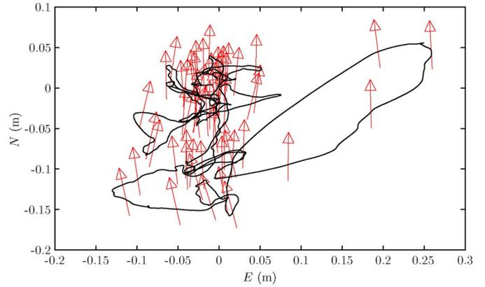
Fig. 12. Horizontal path with airship yaw angle for turbulent gust case.
