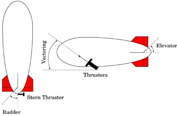
Fig. 1. Airship actuators.
