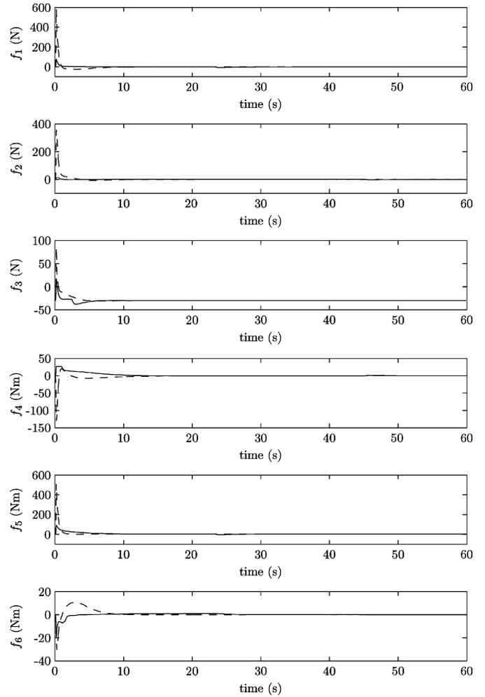
Fig. 5. Control inputs, with full actuation (dashed line) and saturated case (solid line), forces on top and torques below.
