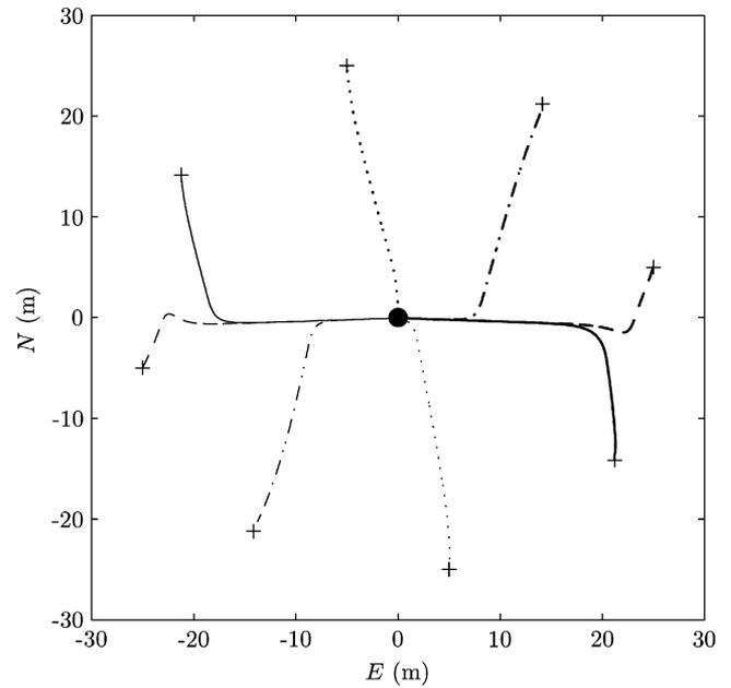
Fig. 8. Horizontal path for different starting points, for saturated forces case.
