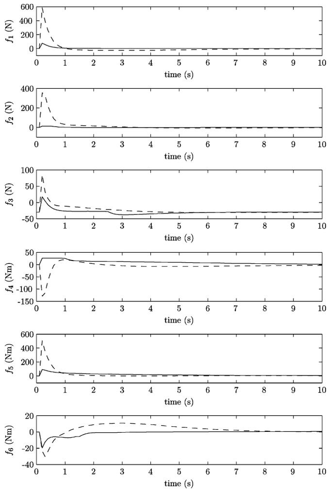
Fig. 6. Control inputs curves zoom, with full actuation (dashed line) and saturated case (solid line), forces on top and torques below.
