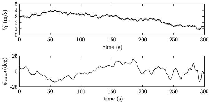
Fig. 13. Airspeed and wind heading estimation for turbulent gust case.
