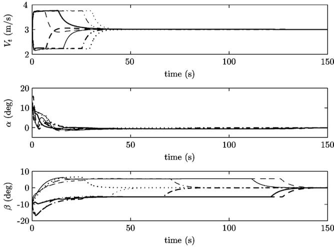
Fig. 10. Airspeed and aerodynamic angles for different starting points, for saturated forces case.
