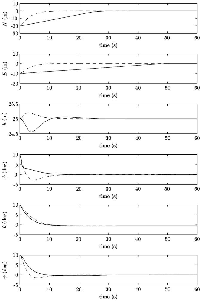
Fig. 3. Position variables, in full forces case (dashed line) and saturated case (solid line) and from top to bottom, the cartesian North-East-Up coordinates, and roll-pitch-yaw Euler angles.
