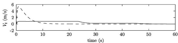
Fig. 7. Airspeed, for full forces case (dashed line) and saturated case (solid line).
