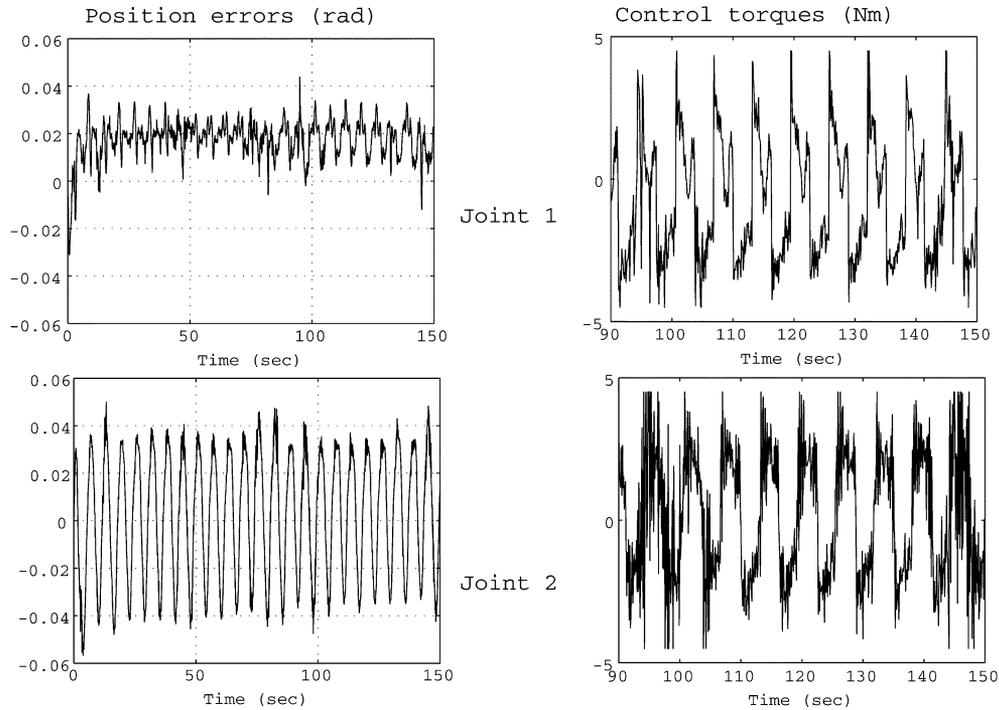
Fig. 5. Experimental results for traditional LP adaptive controller (37): (left) Tracking errors of joints and (right) characteristics of control inputs.
