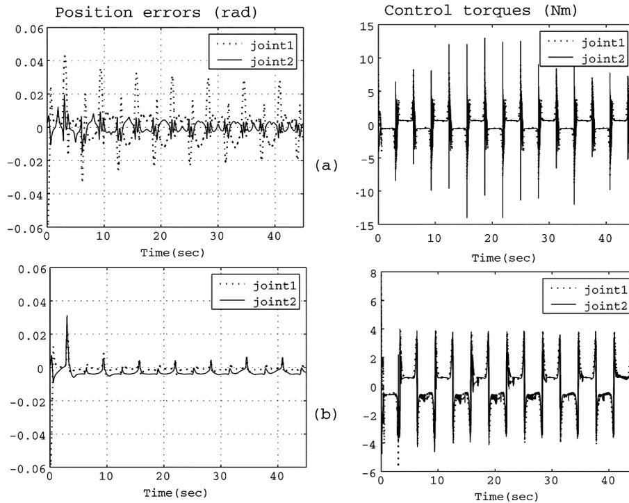
Fig. 3. Simulation results: (left) Tracking errors of joints and (right) characteristics of control inputs. (a) Traditional LP adaptive controller (37). (b) Proposed controller (35).
