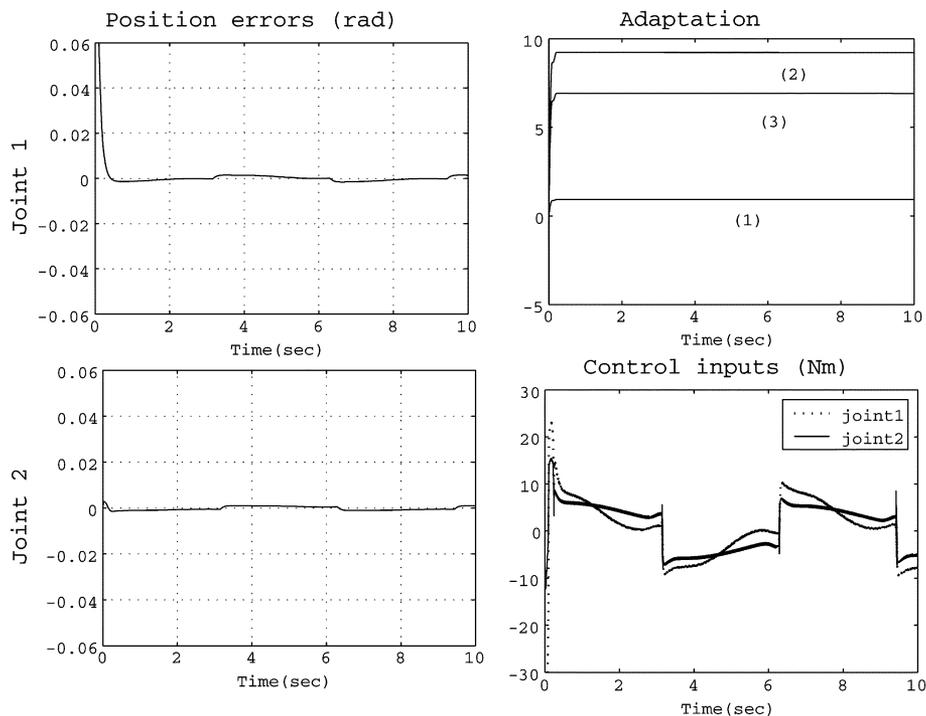
Fig. 4. Simulation results for proposed 1-D-estimators (29): (left) Tracking errors of joints (right) the adaptation of the estimates and characteristics of control inputs. (1)  $\hat{a}$ ; (2)  $\hat{\alpha}$ ; (3)  $\beta$ .
