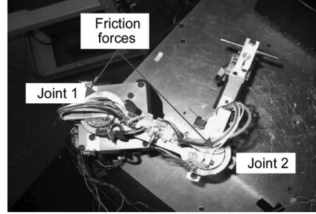
Fig. 2. Prototype of robot manipulator.
