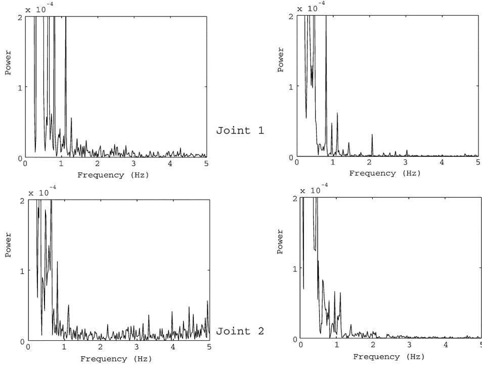
Fig. 9. Experimental results: FFT of trajectory tracking errors for (left) traditional LP adaptive controller (37) and (right) proposed controller (35).
