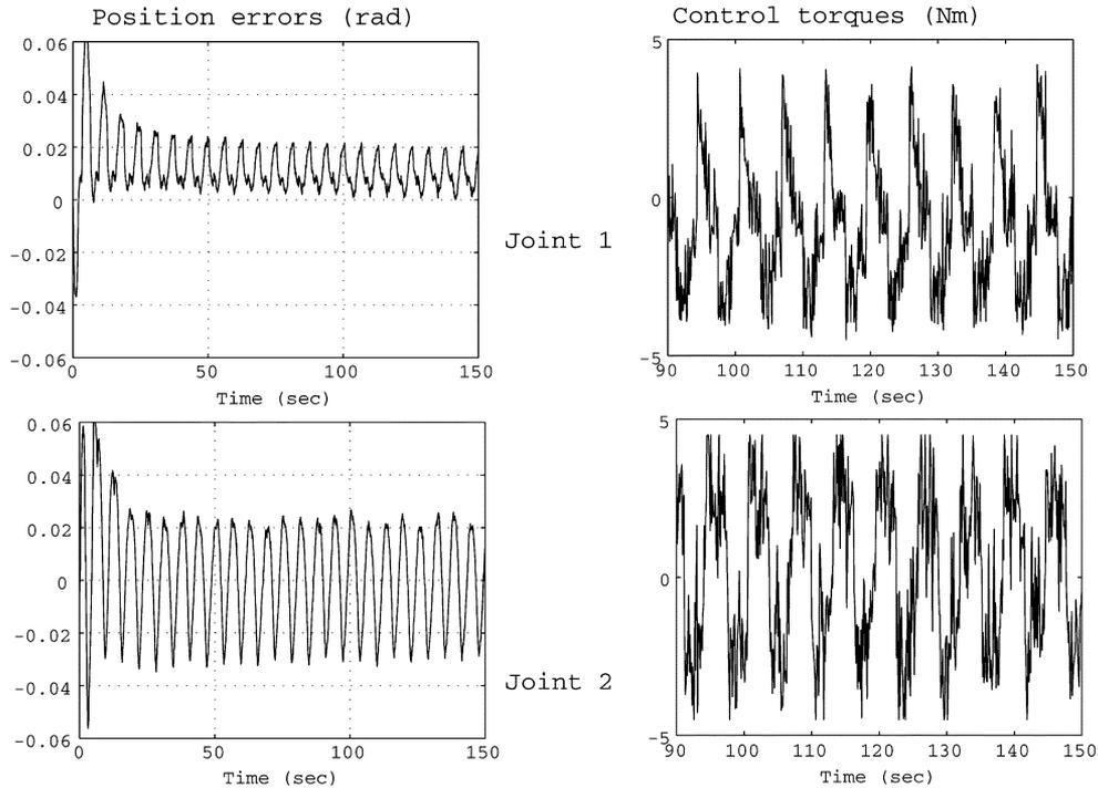
Fig. 6. Experimental results for proposed controller (35): (left) Tracking errors of joints and (right) characteristics of control inputs.
