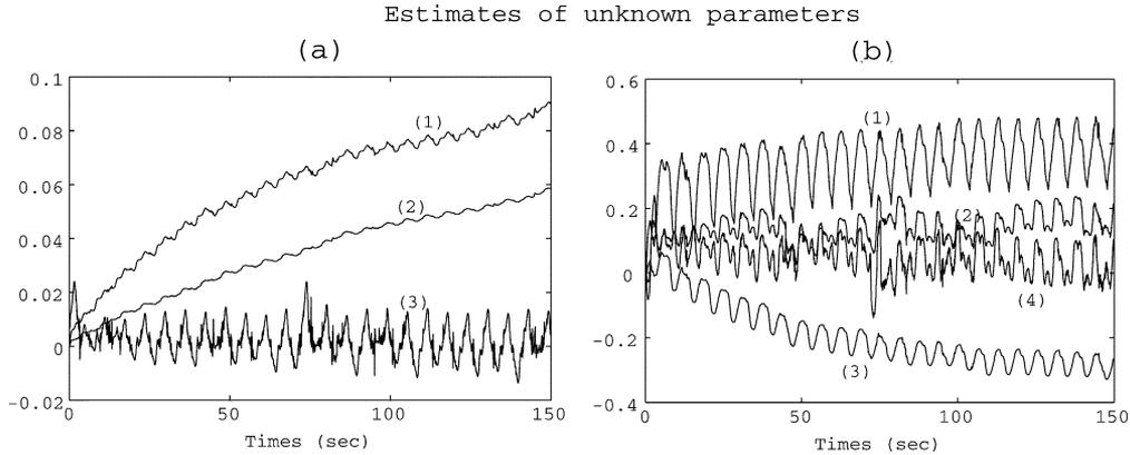
Fig. 7. Experimental results: Estimates of unknown parameters with traditional LP adaptive controller (37). (a) Estimate  $\hat{a}$ : (1)  $-\hat{a}_1$ , (2)  $-\hat{a}_2$ , (3)  $-\hat{a}_3$ . (b) Estimate  $\hat{\alpha}$ : (1)  $\hat{\alpha}_1$ ; (2)  $\hat{\alpha}_2$ ; (3)  $\hat{\alpha}_3$ ; (4)  $\hat{\alpha}_4$ .
