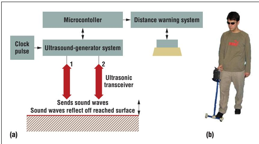
Figure 2. The ultrasonic walking stick: (a) a system diagram and (b) the walking stick in use.
