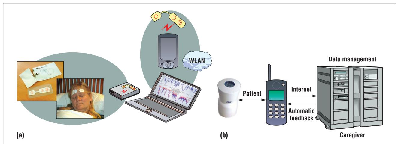
Figure 1. Two applications of the MINAmI project: (a) the ultra-light data logger and (b) the smart pillbox.
