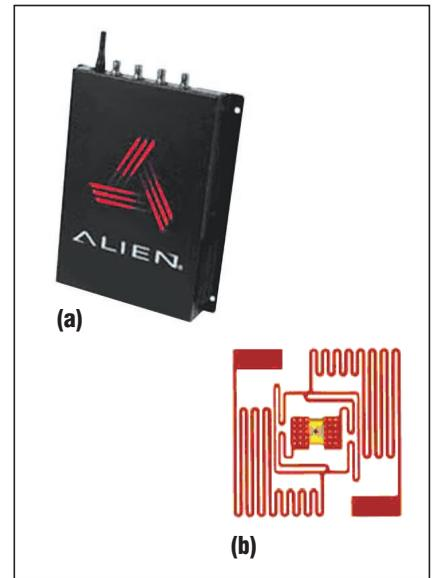
Figure 3. The RFID (a) reader and (b) tag used to evaluate and monitor psychiatric patients.
