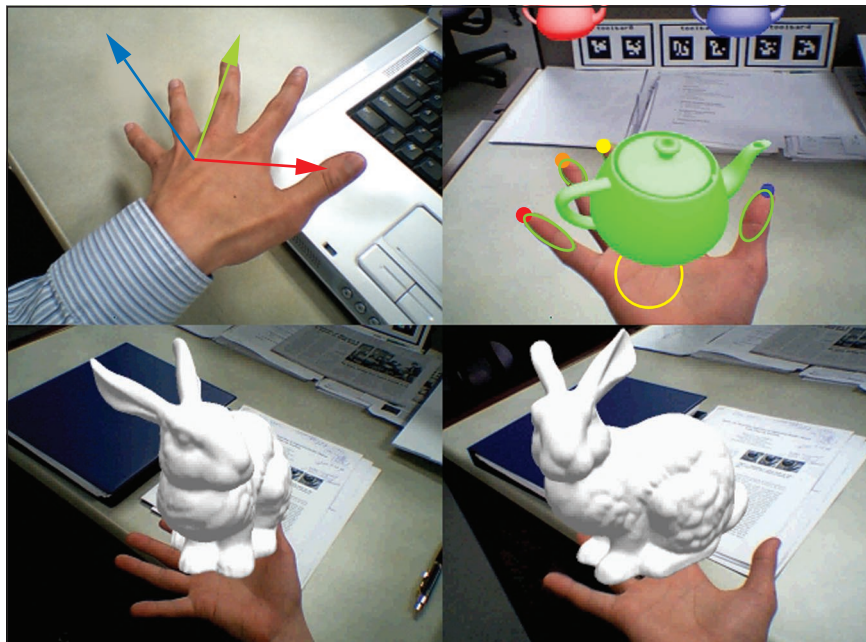
Figure 3. The HandyAR augmented-reality system based on robust hand and fingertip tracking to inspect virtual objects (such as a bunny) on top of the user's hand.
