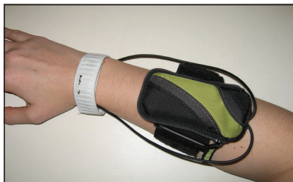
Figure 1. Hambone gesture recognition prototype: sound is generated by hand movements that travel to the device via bone conduction.
