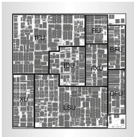
Figure 2. The z10 microprocessor core, organized into eight units. (IFU: instruction fetch unit; IDU: instruction decode unit; LSU: load-store unit; XU: translation unit; FXU: fixed-point unit; BFU: binary floating-point unit; DFU: decimal floating-point unit; RU: recovery unit.)
